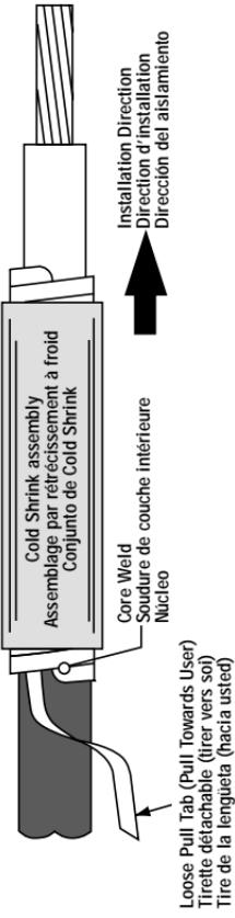
2. Make connection and clean cable insulation 2" (5 cm) minimum.
