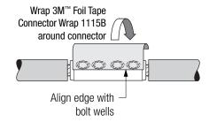
3.8 Once foil tape is properly aligned, continue wrapping the foil tape around the connector until it covers the bolt wells with a second layer. Press down the ends of the tape at the final edge and near the connector tapers.
