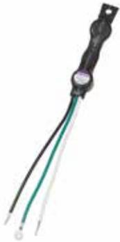
Adapted to SSL outdoor lighting, the Philips SP1HV surge protection device provides single phase protection for line/neutral, line/ground and neutral/ground in accordance with IEEE C62.41 2002 C Low. The SP1HV's small size corresponds to the current design requirements for the new technology luminaires, like an LED light engine in outdoor lighting.
