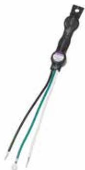
Adapted to SSL outdoor lighting, the Philips SP1 surge protection device provides single phase protection for line/neutral, line/ground and neutral/ground in accordance with IEEE C62.41 2002 C Low. The SP1's small size corresponds to the current design requirements for the new technology luminaires, like an LED light engine in outdoor lighting.
