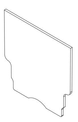
1.) PLATE MATERIAL: POLYCARBONATE 2.) UL LISTED WITH 2 HOUR FIRE RATING 3.)LOW VOLTAGE PLATE FOR USE WITH 2302, 3303, 4304, 5305 SERIES AND 9314 ONLY.
