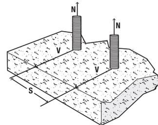
**Edge Distance, Tension ( $F_{NC}$ ) (Lightweight concrete only)**
