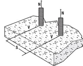
**Edge Distance, Tension ( $F_{NC}$ ) (Normal-Weight concrete only)**
