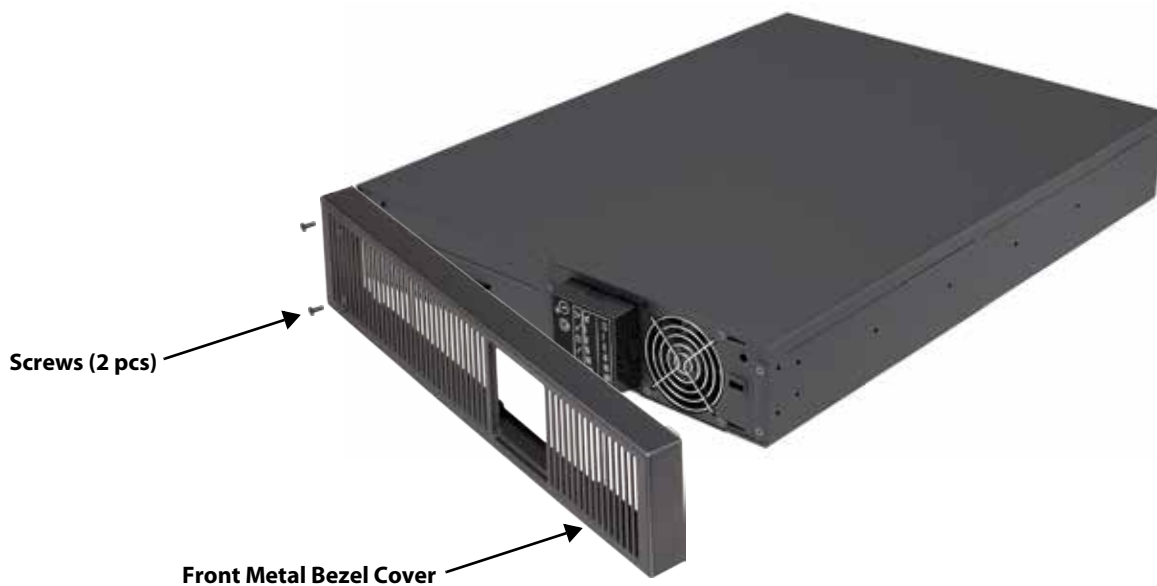
Figure 5: Remove the front metal bezel cover
