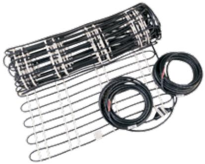
**H-Mat** – H-Mats are custom sized snow/ice melting mats. They are available in outputs up to 72 watts per square foot and in voltages up to 480 Vac. H-Mats are supplied with standard 10-foot cold leads. H-Mats are UL Listed. Please contact your local EasyHeat representative for details.
