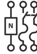
Fusible, Two-pole, 120/240 and 240 Volts AC; 250 Volts DC; Three-wire switching neutral, 240 Volts AC
