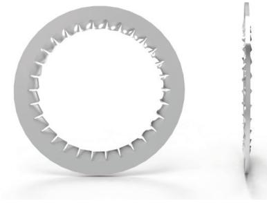
High quality metallic serrated washers designed to protect against loosening of cable gland or locknut in vibrating applications. Often used when mounting a cable gland mounted to a thin wall enclosure, fitted internally with a locknut.
