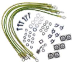
The Grounding Kit allows a PROLINE or PROLINE G2 enclosure to be grounded to VDE specifications. Includes six 12-gauge wires 411 mm (16.19) long with ring terminations and M6 mounting hardware.
