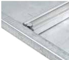
Panel Support Braces give additional support to single- and double-bay panels in heavy loading applications and minimize the vibration created by components mounted on the panel. Braces can be installed on existing systems without removing the panel. Panel support braces are furnished in pairs. Braces are unpainted galvanized steel.
