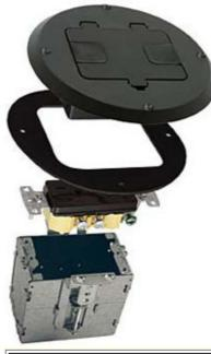
Decorator duplex receptacle floor box kit; includes steel box, flange and hinged door cover assembly with 15Å 125V tamper-resistant duplex receptacle; designed for installation in wood floors; mounts to subfloor or ioists
