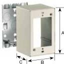
For deep devices (such as momentary contact switches) or applications where additional room is beneficial. Single gang box base has two  $\frac{1}{2}$  in. trade size KOs. Two gang box base has a rectangular KO and concentric  $\frac{1}{2}$  in. and  $\frac{3}{4}$  in. trade size KOs. Three gang box base has one  $\frac{1}{2}$  in. trade size KO per gang.
