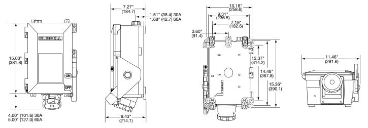
Note: 30A – 1 inch NPT hub supplied; 60A – 11/4 inch hub supplied.
