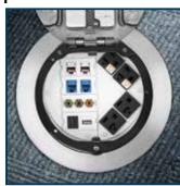
**50/50 6 Inch Sub-Plate Split** Two duplexes with ample audio/video and data are achieved by using the 50/50 sub-plate layout. Additionally this layout will accommodate two Style Line<sup>®</sup> devices for GFCI, surge, etc. applications. 6 Inch Recessed Access
