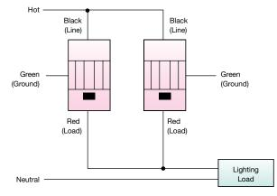
Note: \* Load can not exceed the rating of one switch.
