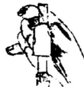
4. Insert conductor all the way into the barrel of the CPM adapter.
