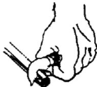
2. Strip the wire insulation using an approved method. Do not nick or ring the conductor. Be sure and remove any mylar coating on the wire.
