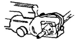
5. Select the proper die for approved tool. See chart above for approved tools and dies. Compress from copper pin toward conductor at the first inked line. Remove flash and excess De-ox before slipping provided cover in to place.
