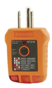
Klein Tools Receptacle Testers are designed to detect the most common wiring problems in standard and GFCI receptacles. A convenient chart on the tester helps determine wiring condition in outlet, based on LED lights results. Conditions indicated: open ground, reverse polarity, open hot, open neutral, hot/ground reversed.
