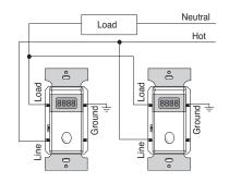
When using a three-way application, lights may be turned on from either switch, but can only be turned off at the switch that turned them on.
