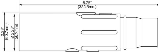
Taper Nose In-line Latching Female Plugs - Vulcanized
