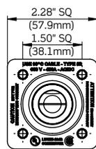
Typical for Bus Bar Termination (Top View)
