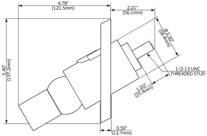
Mounting Pattern Common to Both Male & Female Configurations
