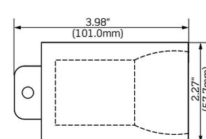
**23 Series Latching Taper Nose Plugs - 690A, 600V Max**
