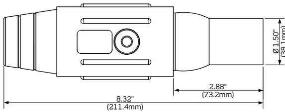
Ball Nose In-line Latching Female Plugs S-Series
