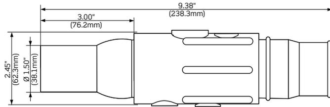
Ball Nose In-line Latching Male Plugs S-Series
