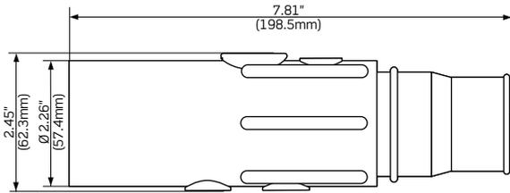
Ball Nose In-line Latching Female Plugs
