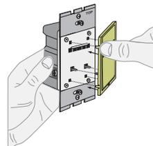
Line up and insert right side tabs, then rotate left to attach new face
