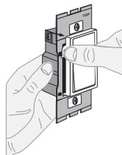
Push in sides at tabs and pull to release face
