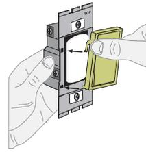
Attach new face by inserting the bottom hinge tabs, then pivot and snap on the new face
