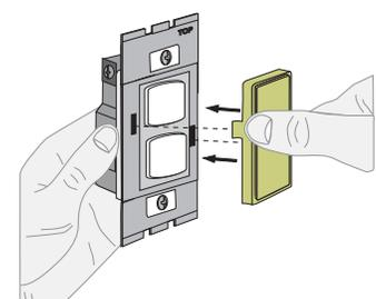
Insert right side tab and rotate left to attach
