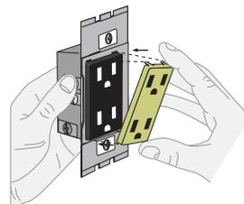
Attach new face by inserting bottom hinge tabs, then pivot and snap on the new face
