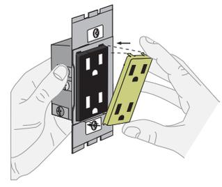
Attach new face by inserting bottom hinge tabs, then pivot and snap on the new face
