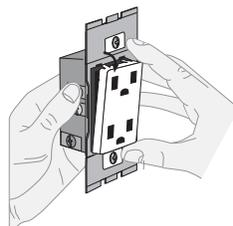
Push down tabs per diagram, one at a time and rotate forward to release face
