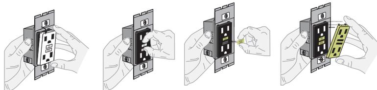
Push down tabs per diagram, one at a time and rotate forward to release face
