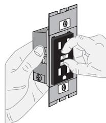
Pull out Test and Reset buttons
