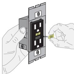
Insert new Test and Reset buttons
