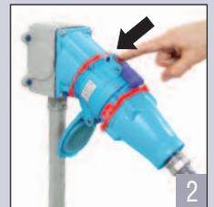
Pressing the pawl causes the DECONTACTOR to break the circuit. The plug is ejected to its rest position; its contacts are now dead.
