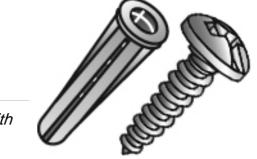
Conical anchors are designated by the size screw they are used with and the length which is measured from end to end.
