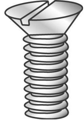
*A straight shank fastener with external threads designed to go through a hole or nut that is pre-tapped to form a mating thread for the screw.*
