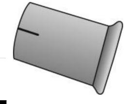
A two-piece, internally threaded expansion anchor with four equallyspaced longitudinal slots extending from the bottom end of the outer shield, inside of which sits a pre-assembled dilating plug.
