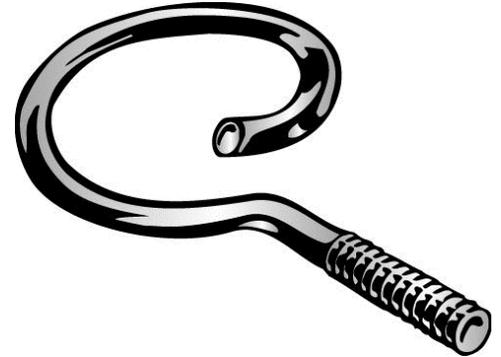
*The cable bridle ring's design allows for cables to be added or removed at any time due to the "corkscrew" ring which allows access space for adding or removing cables and at the same time providing 360° degrees capturing of the cable or bunch of cables.*
