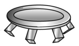
Snap-in style knockout seals are inserted in discontinued, open box knockouts to protect exposed wires.
