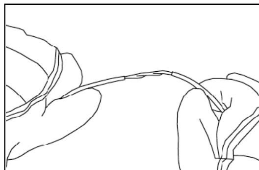
Removing the outer length of the simplex jacket
