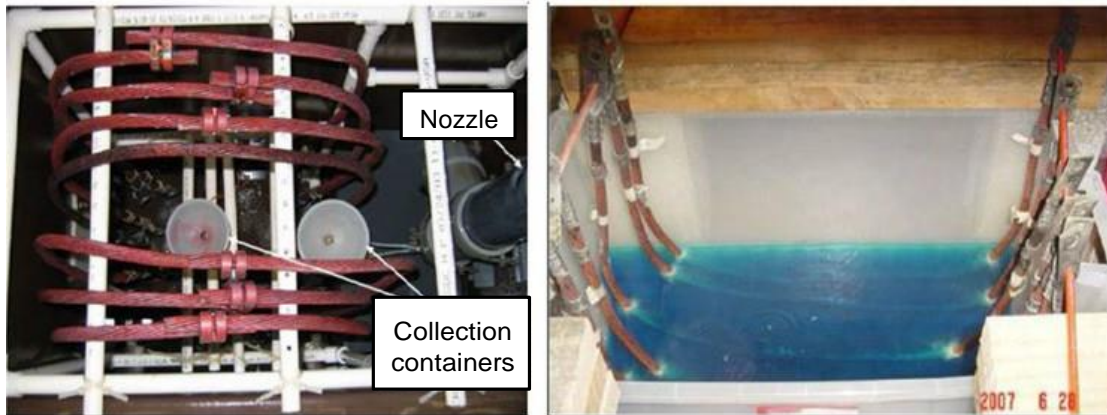
Figure 6. Testing set-up for salt spray (left) and acid bath (right) sequence tests.
