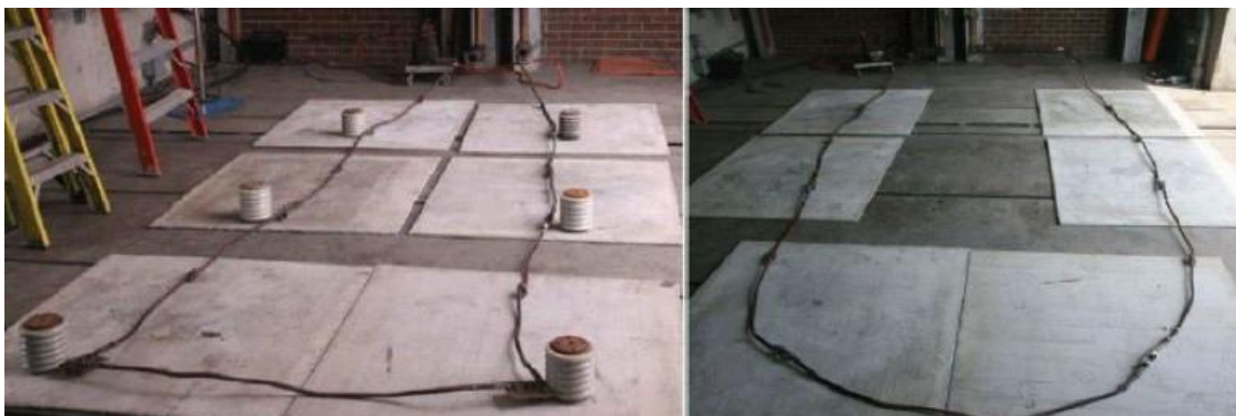
Figure 7. Fault current test layout for the acid sequence and salt spray samples.
