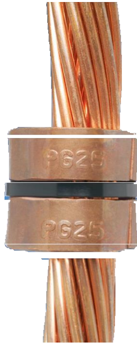
Figure 10. Isolated view of Panduit GCE250-250 with IEEE 837 die number embossment verification.
