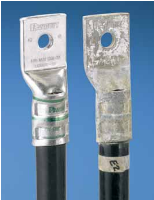
Before and after rigorous NEBS Level 3 testing.
