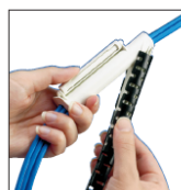
Slide Pan-Wrap™ Split Harness Wrap onto end of tool until approximately 3" of it covers the bundle.
