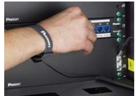
Figure 4. ESD wrist straps and ports enhance equipment protection.
