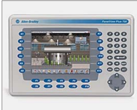
Figure 4: Image of the PanelView™ Plus 6 700 Graphic Terminal
