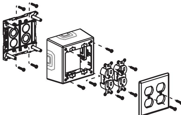
The mounting hardware used to secure the base shall be appropriate for the mounting surface
