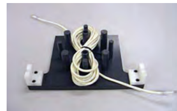
Patch cord rotated on one end on the coil ellipse by 180° to form a figure eight cable loop, up to 10 loops total.
