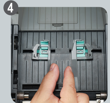
Use fingers to widen guides by pressing out
