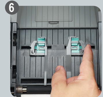
When changing from terminal block markers to other types of labels, use the rear tabs on the width guide inserts to lift and remove them from the green printer guides
