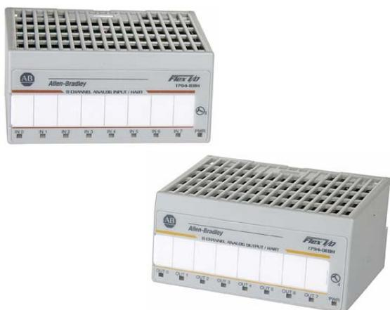
The FLEX I/O module plugs into the terminal base, connecting to the I/O bus and field devices. Since there is no direct wiring to the I/O module, you can remove and insert modules under backplane power, enabling you to change modules without disturbing field wiring, other I/O modules, or FLEX backplane power.
