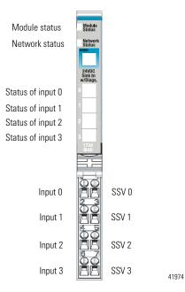
Note: Voltage and current are daisychained from either the adapter, 1734-FPD module, or 1734-EP24DC module.
