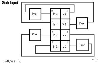
If a common connection is required (three-wire devices), then a 1734-CTM common terminal module can be required.
