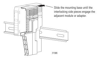
Press firmly to seat the mounting base on the DIN rail until the mounting base snaps into place.
