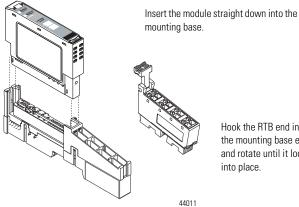
Hook the RTB end into the mounting base end and rotate until it locks into place.
