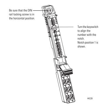
To install the module, use this procedure:
