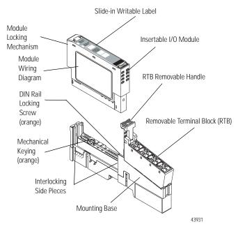
The wiring base assembly includes terminal base, 1734-TB or 1734-TBS, which consists of mounting base, 1734-MB, and removable terminal block. 1734-RTB or 1734-RTBS
