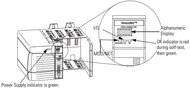
When you apply chassis power, the alphanumeric display cycles through the following information:
