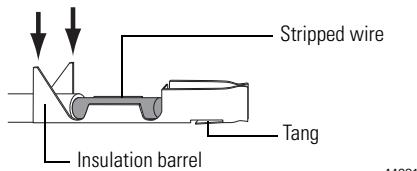
5. Solder wire and wire barrel together using lead-free solder and soldering pencil.
