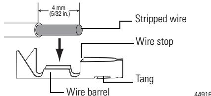
3. Crimp the wire barrel around the wire using small needle nose pliers.
