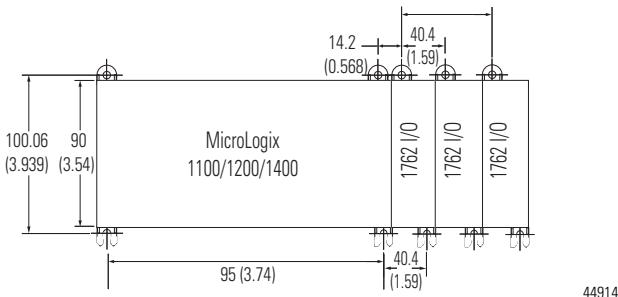
**NOTE:** All dimensions are in mm (in.). Hole spacing tolerance:  $\pm 0.4$  mm (0.016 in.).
