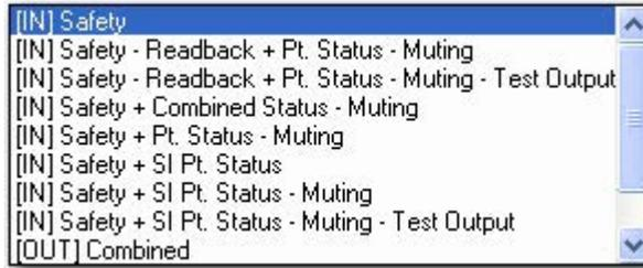
To see the specific data that will be generated for each connection name, in the 1791DS module properties dialog box click the Safety I/O tab. Expand each choice to see the tags created for input data, input status, output data, and output status.
