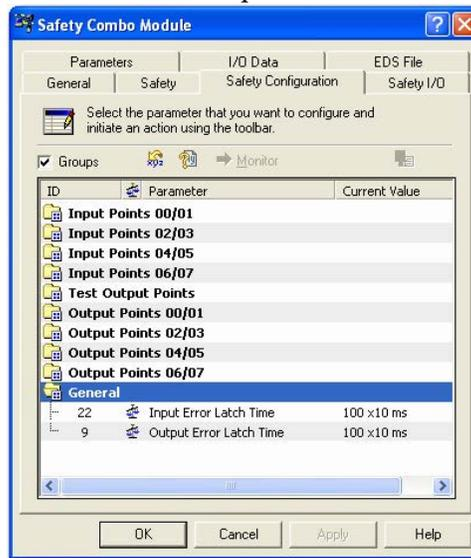
2. Enter the Input Error Latch Time, the time the module holds an error to make sure the controller can detect it (0...65,530 ms, in increments of 10 ms—default 1000 ms).
