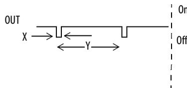
When the external input contact is closed, a test pulse is output from the test output terminal to diagnose the field wiring and input circuitry. Using this function, short-circuits between input signal lines and the power supply (positive side), and short-circuits between input signal lines can be detected.
