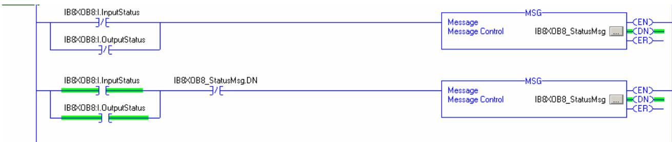
This figure shows the MSG instruction parameters for reading Instance 803 from the 1791DS-IB8XOB8 module.
