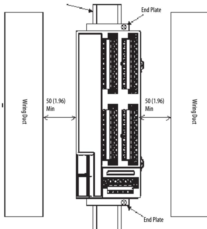
**Figure 22 - Module Installation**
