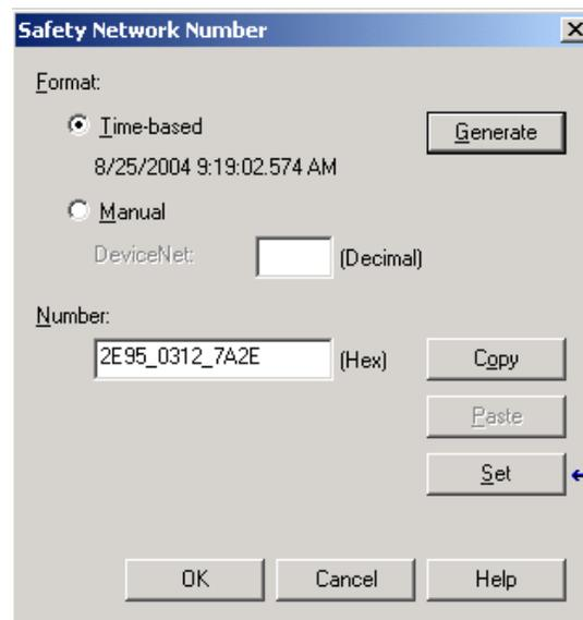
If the project is configured as ‘Configure Only When No Safety Signature Exists’, follow the appropriate steps to replace a Guard I/O module based on your scenario.
