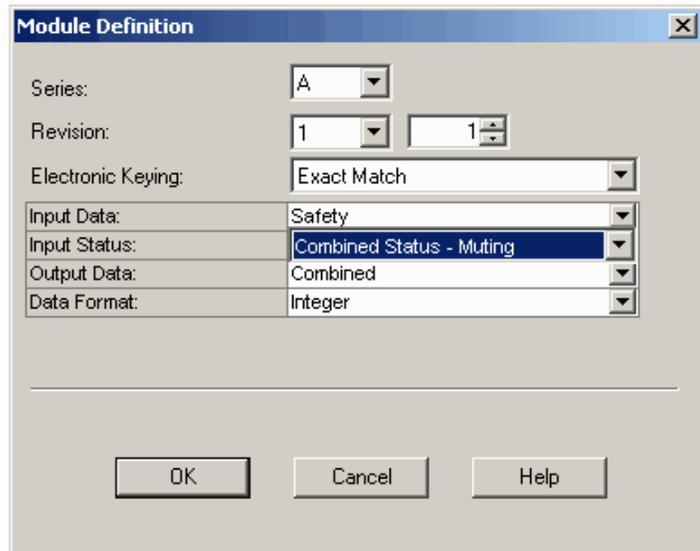
This creates a 2-byte assembly, as shown for the 1791DS-IB12 module.
