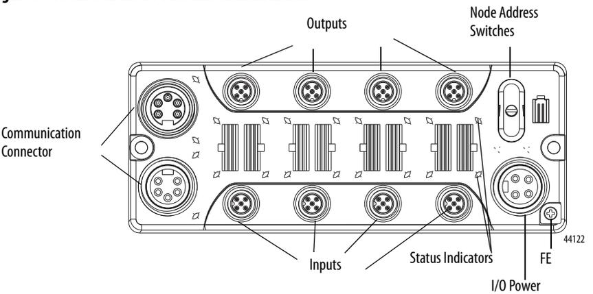
**Figure 9 - 1791DS-IB16 Module Identification**
