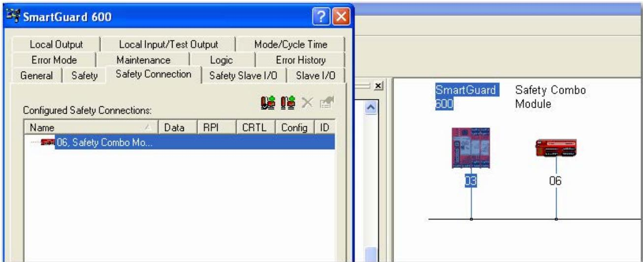
The rest of these steps assumes that the module is a combination input and output module. We describe how to add two connections: one of inputs and one of outputs. You can add individual safety connections for the inputs and outputs. SmartGuard 600 controller can have as many as 32 connections.
