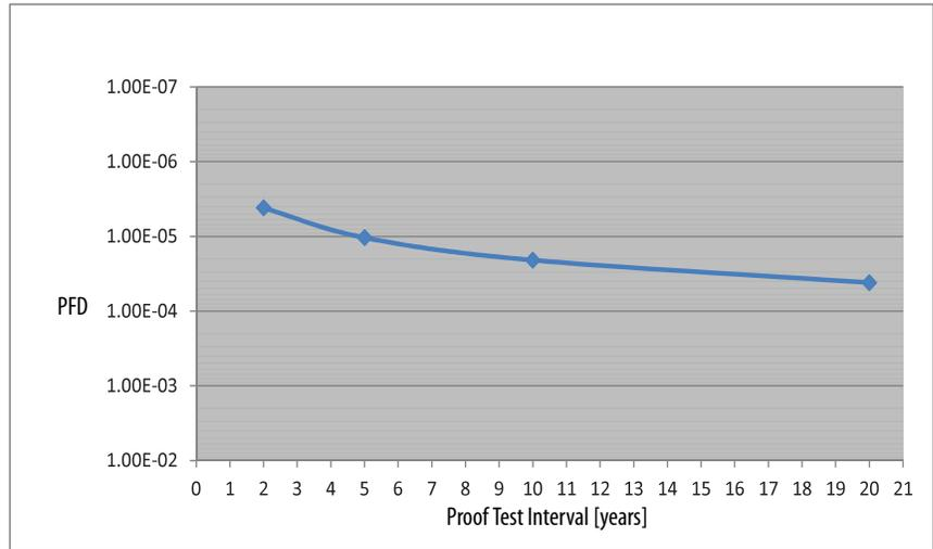
Figure 31 - PFD versus Proof Test Interval 1791DS-IB12, 1791DS-IB8X0B8, 1791DS-IB4X0W4
