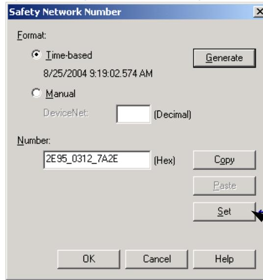
**Figure 28 - Setting the SNN with a SmartGuard Controller**
