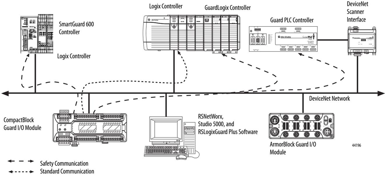
Safety controllers control the safety outputs. Safety or standard PLC controllers can control the standard outputs.
