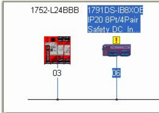
The exclamation point means the SNN has not been set (as shown below). This makes sense because the device has just been reset.
