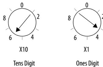
1. Set the node address by using the two rotary switches on the front panel of the module, noting that the default setting is 63 and a value between 00...63 is valid for proper use.
