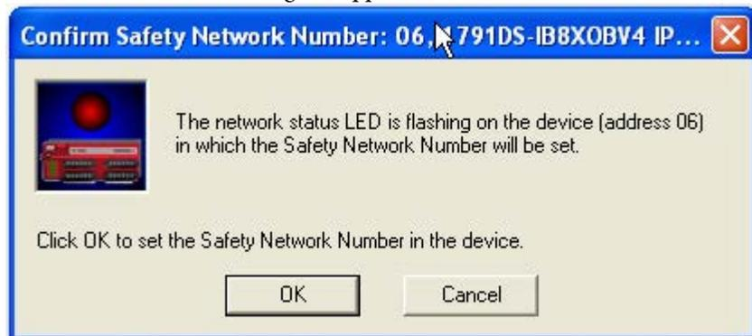
This lets you confirm which 1791DS module is about to have its SNN set. The network status indicator on the module that is about to have its SNN set is flashing red/green. Click OK to confirm the set.
