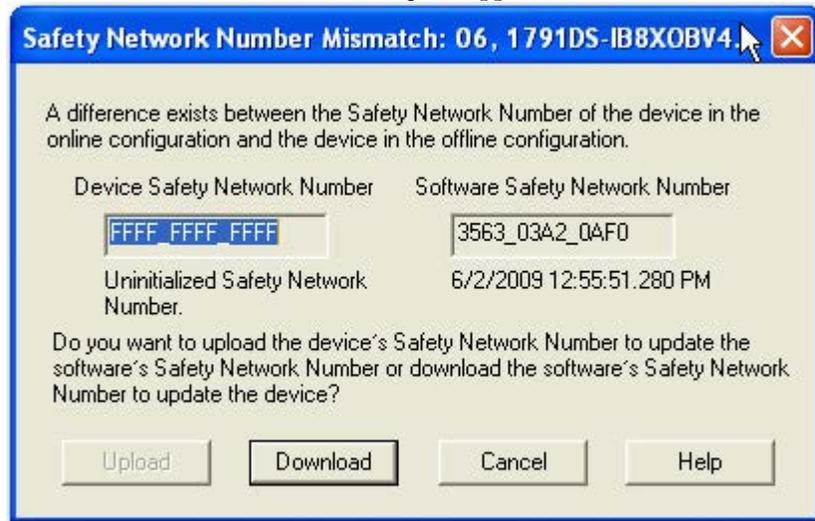
The SNN that exists in the 1791DS module does not match what is in RSNetWorx for DeviceNet software. For more information about the SNN, see [83](#).
