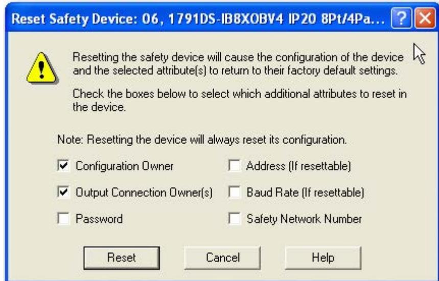
Check Password and Safety Network Number so that the 1791DS module is totally reset. Click Reset.
