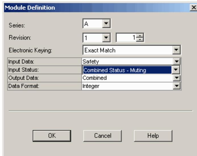
This creates a 2-byte input assembly, as shown for the 1791DS-IB8XOB8 module.
