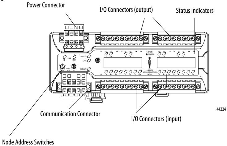
**Figure 7 - 1732DS-IB8 Module Identification**
