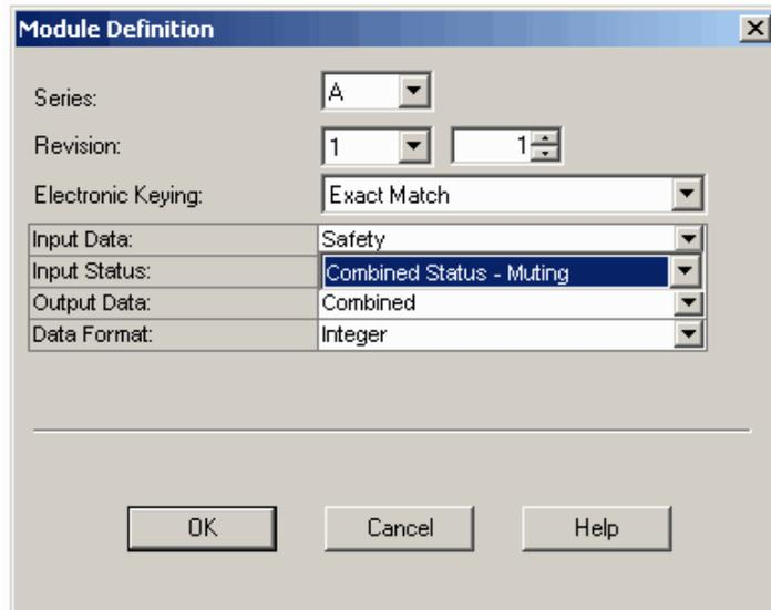
This creates a 1-byte input assembly, as shown for the 1791DS-IB4XOW4 module.
