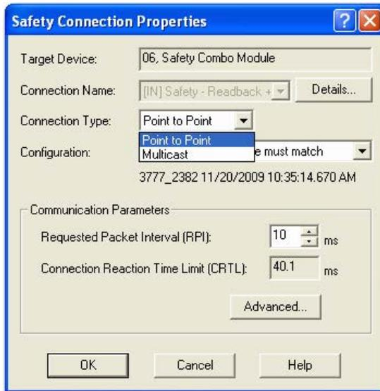
The Multicast connection type enables other safety controllers to read the safety input data by using this input connection. The Point to Point connection type does not enable this functionality.
