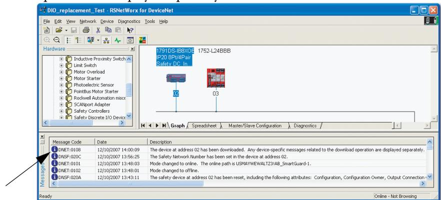
Assuming this is the proper configuration from the original DNT file, the SNN and configuration signature now match that of the original. If you are already connected to the SmartGuard controller, a connection is made. The SmartGuard controller does not need to be taken out of RUN mode to download to the replacement module.
