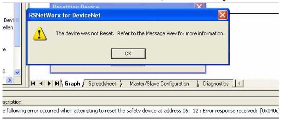
Put the SmartGuard controller into Idle mode and attempt to reset the 1791DS module again.
