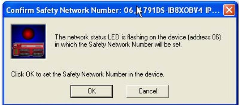
The network status indicator on the module that is about to have its SNN set is flashing red/green.
