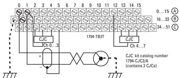
**IMPORTANT** When using grounded thermocouples, and the error is off the same amount on each thermocouple, connect terminal 16 to ground, and connect the thermocouple ground to the same ground.
