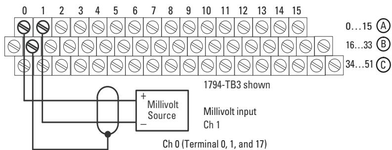
For more accurate readings, use the 1794-TB3T for mV measurement.
