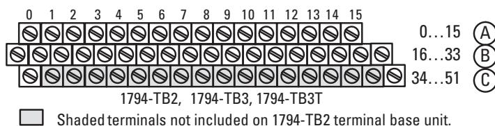
**IMPORTANT** Use 1794-TB3T or 1794-TB3TS terminal bases for thermocouple or millivolt inputs.
