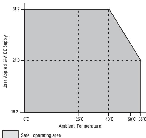
The area within the curve represents the safe operating range for the module under various conditions of user supplied 24V DC supply voltages and ambient temperatures.
