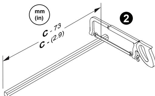
**Typical Operating Shaft Installation**
