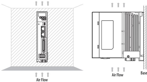
**IMPORTANT** Mount the drive in an upright position, as shown. Do not mount the drive horizontally (that is, rotated 90 degree from the upright position) or with front cover facing upward or downward.
