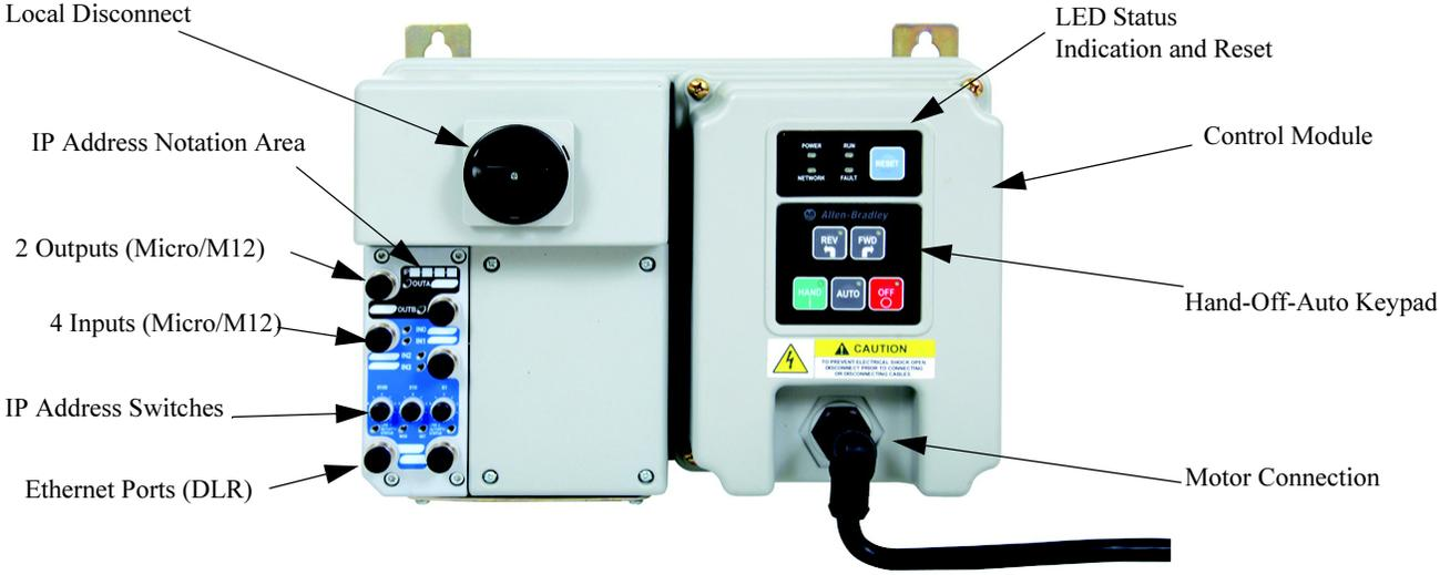
Figure 11 - Bulletin 284E ArmorStart with EtherNet/IP Communication Protocol
