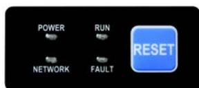
The Control Module LED status and diagnostics consists of four status LEDs and a Reset button. The following is a brief explanation of the operation of each LED found on the Control Module.
