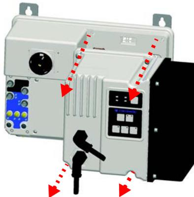
Figure 25 - Bulletin 284E Jumper Removal
