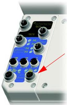
EtherNet/IP LED status and diagnostics consists of four LEDs.
