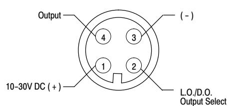
Selection of the output state: (white wire must be connected for operation): L.O. (White –), D.O. (White +)
