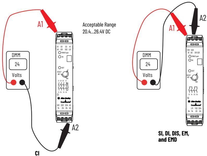
If the voltage is not within the acceptable range, verify that the power supply, wiring, circuit breakers, and/or fuses are functioning properly.
