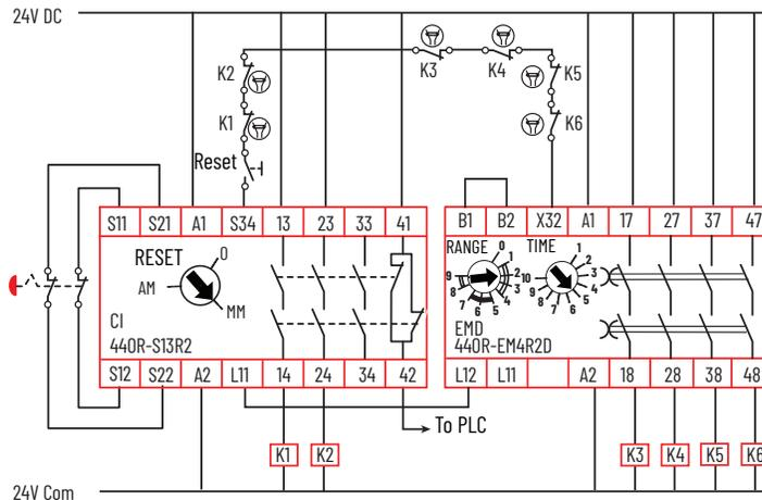
[Figure 51 on page 49](#) shows the EMD safety relay that is configured for a 2.1 second on-delay. The single wire safety signal from terminals L11 to L12 instructs the EMD safety relay to turn on and off. When the Reset button is pressed, the DIS safety relay outputs turn on immediately. After a 2.1 second delay, the EMD safety relay outputs turn on.
