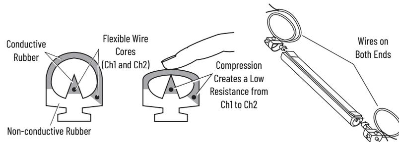
Figure 15 on page 24 shows the typical wire connections. With the proper connection, GSR safety relays detect the compression of the edge and turn off their outputs. With no pressure on the edge, the GSR outputs can turn back on with a reset signal.
