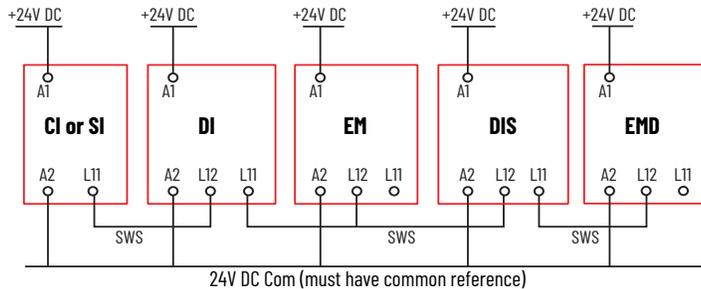
Figure 20 shows the characteristics of the SWS signal when it is active. It starts with a 1 ms pulse, followed 700  $\mu$ s later by a 500  $\mu$ s pulse. This waveform is repeated every 4 ms. When inactive, the SWS is 0V.
