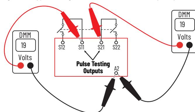
2. Check the voltage at each of the inputs with the device contacts closed, as shown in [Figure 63 on page 59](#). The values must be very close to the values measured at terminals S11 and S21.
