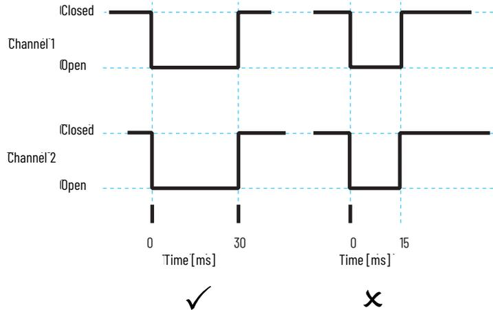
Fast input cycling, where both input channels are cycled simultaneously, has three outcomes:
