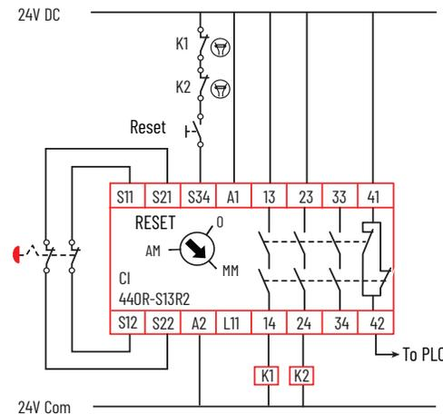
[Figure 44 on page 46](#) shows a CI safety relay monitoring a safety light curtain with two OSSD outputs. The CI safety relay is set to automatic/manual reset (AM). The auxiliary signal (terminals 41/41) informs the PLC that the safety system is off or on. The CI safety relay outputs connect to AC voltage loads. When the CI safety relay is on, the PLC can then turn on the K1 and K2 contactors.
