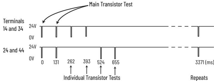
Although pulse tests appear on terminals 34 and 44, the DIS safety relay does not detect faults from A1 to 34, 44 or between 34 and 44 when the outputs are on.
