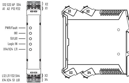
Figure 6 shows the markings on the front face of each safety relay, including the terminal and status indicator identifications.
