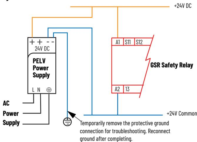
IEC 60204-1 edition 5.1 (Section 6.1) allows a SELV supply to be used when a PELV is not practicable due to physical or operational conditions. NFPA79 does not allow the use of a SELV supply. If you are meeting only IEC 60204-1, you can install a separate SELV supply for your safety system and leave it ungrounded (no protective ground).
