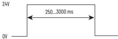
You can create the signal with a momentary push button or programmatically create the signal with a logic controller. [Figure 24](#) shows example wire connections for the reset. The schematic also shows an example monitoring the mechanically linked, normally closed contacts of two contactors.
