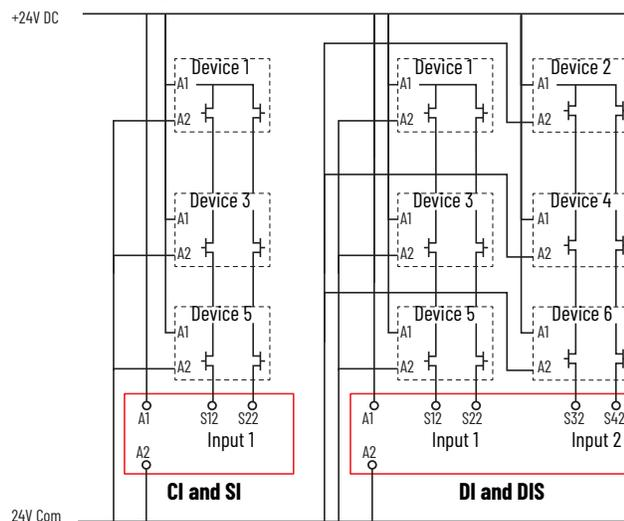
GSR safety relays cannot detect short circuits of the OSSD device outputs. The PWR/Fault status indicator of your GSR safety relay remains steady green. The device with the OSSD outputs must detect short circuits of its own OSSD outputs. When detected, the device must shut off both OSSD outputs and go to a faulted state. A status indicator must inform you that the OSSD is faulted.
