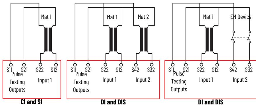
Because the safety mats are parallel plates, they have a significant capacitive effect. The larger the safety mat, the more capacitance. If the capacitance is too large, the safety relay does not function properly. See [Capacitance Effect on page 61](#) for further information.
