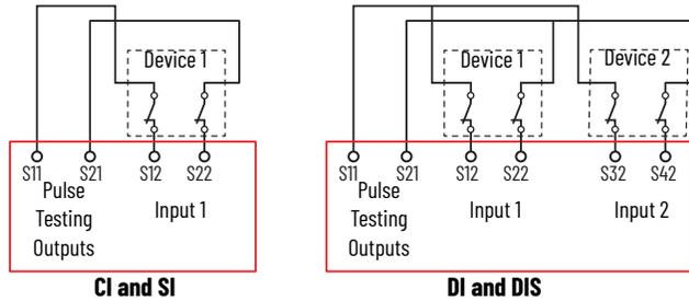
Figure 9 shows the typical connections for devices with 1 N.C. mechanical contact. One side of the contact is connected to a pulse-testing output S11. The other side is connected to two input terminals. The CI and SI safety relays only have one set of input terminals. The DI and DIS safety relays have two sets of input terminals. The DI and DIS safety relays can operate with only one device that is connected or with devices that are connected to both inputs.
