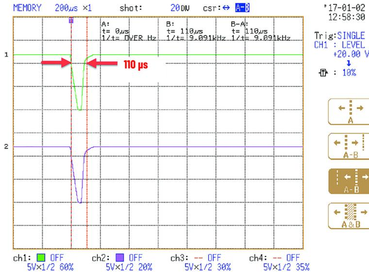
Figure 85 - OSSD Channel Transistor Test Pulse
