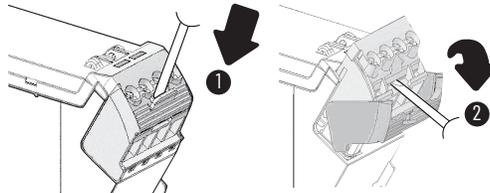
1. Insert the tip of a small screwdriver into the slot near the terminal screws.
