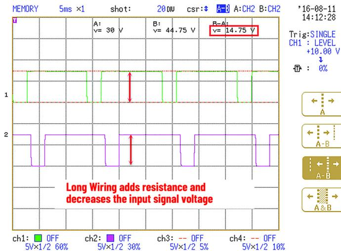
GSR safety relays have a maximum input resistance of 900 ohms.
