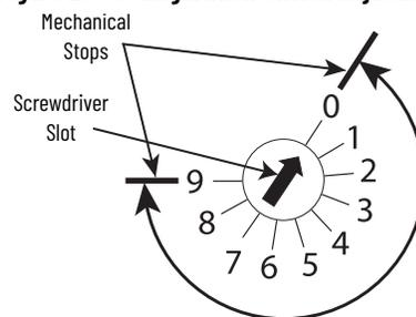
**IMPORTANT** Adjust the switches gently and do not turn past the mechanical stops.
