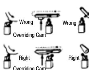
Cam or dog arrangements should be such that the actuator is not suddenly released to snap back freely.
