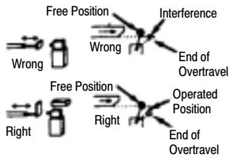
Operating mechanism for limit switches should be so designed that under any operating or emergency conditions the limit switch is not operated beyond its overtravel limit position. A limit switch should not be used as a mechanical stop.
