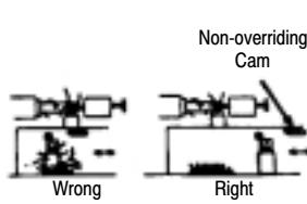
Limit switches should be placed in locations where machining chips do not accumulate under normal operating conditions.
