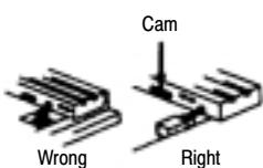
Limit switches should be mounted rigidly and in readily accessible locations with suitable clearances to permit easy service and replacement when necessary. Cover plates should face the maintenance access point.
