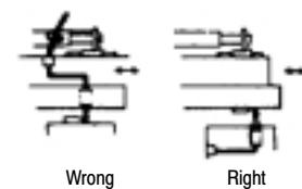
The location of oiltight limit switches and the method of connecting them should be such that condensation in the conduit cannot enter the switch enclosure.
