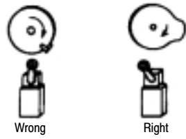
Where relatively fast motions are involved cam arrangements should be such that the actuator does not receive a severe impact. Cams should be designed such that the limit switch will be held operated long enough to operate relays, valves, etc.
