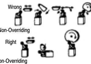
For limit switches with lever actuators, the actuating force should be applied as nearly perpendicular to the lever as practical and perpendicular to the shaft axis about which the lever rotates.
