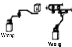
Limit switches are designed for proper performance with the actuators with which they are supplied. Supplementary actuators should not be used unless the limit switches are specifically designed for them.
