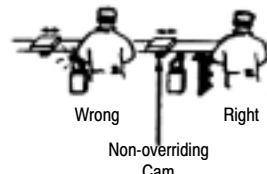
Limit switches should be mounted in locations which will prevent false operation by normal movements of operator or machine components.
