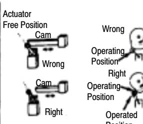
A limit switch actuator must be allowed to move far enough for positive operation of the contacts.
