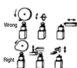
For limit switches with pushrod actuators the actuating force should be applied as nearly as possible in line with the pushrod axis.
