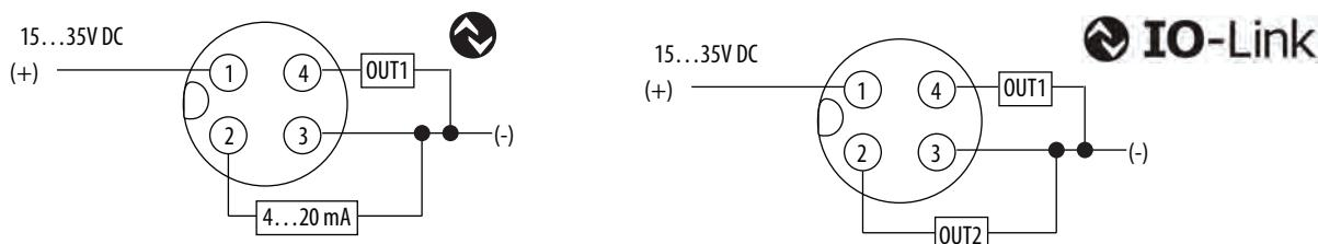
**IMPORTANT** IO-Link operation is only available when connected to an IO-Link Master such as the 1734-4IOL or any competitive IO-Link Master. While in Standard IO mode (SIO), the sensor operates as a discrete PNP output.
