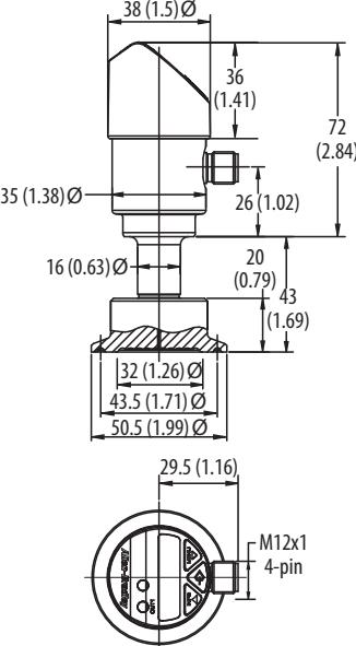
The technical drawing provides detailed dimensions for the 1.5 in. tri-clamp process connection. Key dimensions include:
