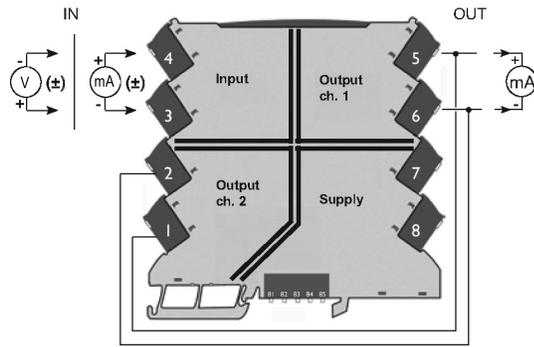
**IMPORTANT** Splitter function is not available when bipolar output function is used.
